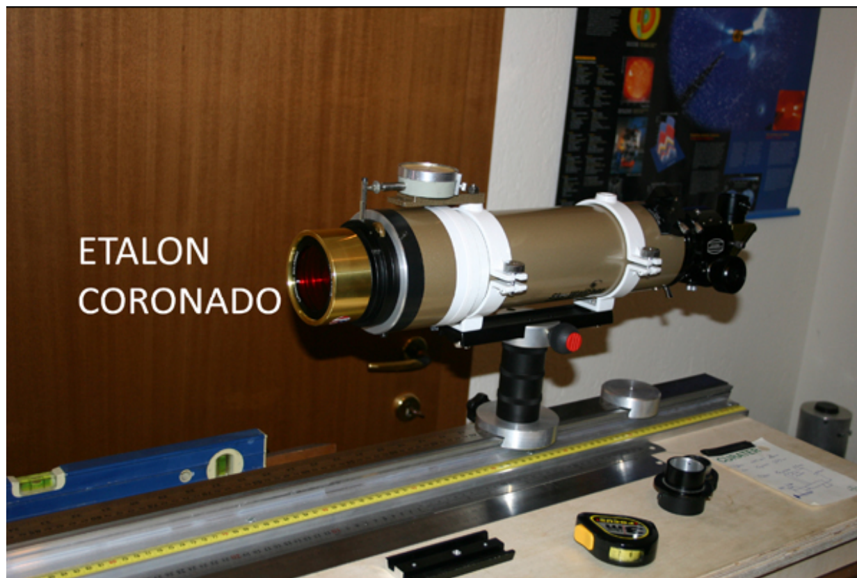
Image 1: The etalon of the Coronado 60 adjusted to a Skywatcher ED 80
